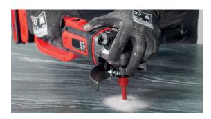
It will be necessary to make a previous hole with a specific drill for hard materials, such as porcelain, with a minimum diameter of 10mm, then a specific disc for these materials will be used and thus join those holes on the outside. We must not go beyond the outside of the circumference, since we would not achieve the end we are looking for.
