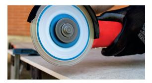
On the other hand, if we opt for a high quality finish cut, mitering or beveling, we can use an electroplated diamond blade such as RUBI's **ECD**.
