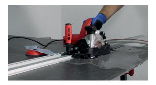
Electric cutting can be done it with a dry diamond blade or a wet cut with a specific blade for this purpose.
